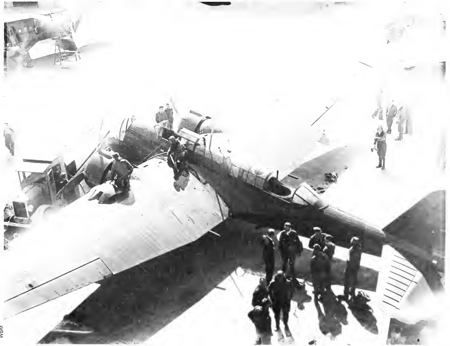
A Martin B-10 bomber being serviced and refueled at the Cheyenne airport on April 19, 1934. The B-10 usually carried a three man crew to include pilot, navigator/bombardier in front bubble, and gunner in back cockpit. When carrying the air mail, the B-10 usually had one or two crew members with the mail loaded in the bomb bay and crew compartments. Note the heavy flying clothes worn by the crew members.
